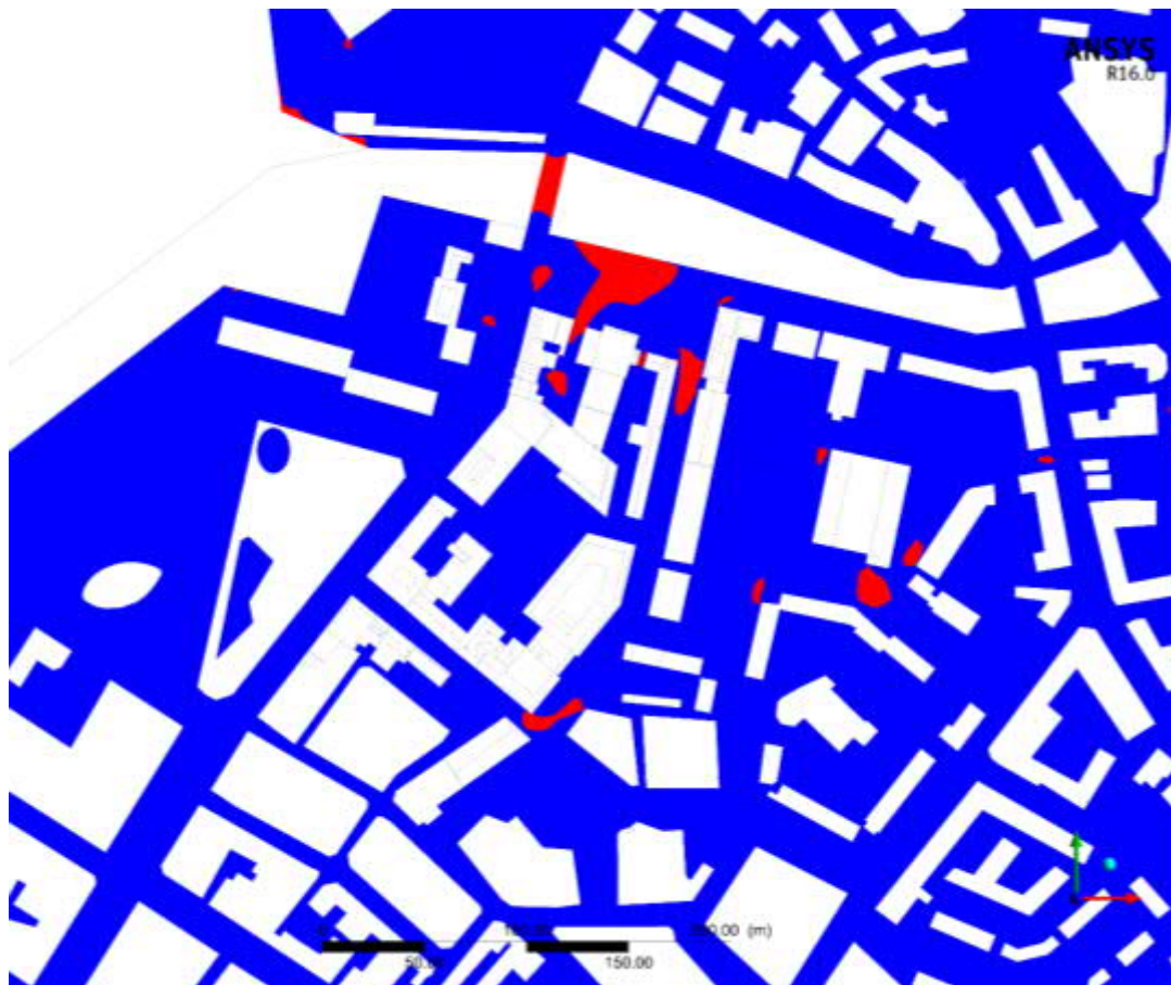
Figure 11-16: Lawson 15m/s Distress for frail/elderly and cyclists - Proposed development. Red indicates unacceptable conditions.
