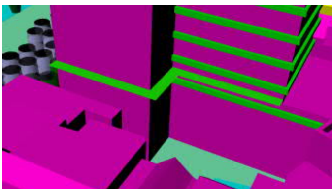
Figure 11-21: Mitigation Measure 2 – Tower Skirt
