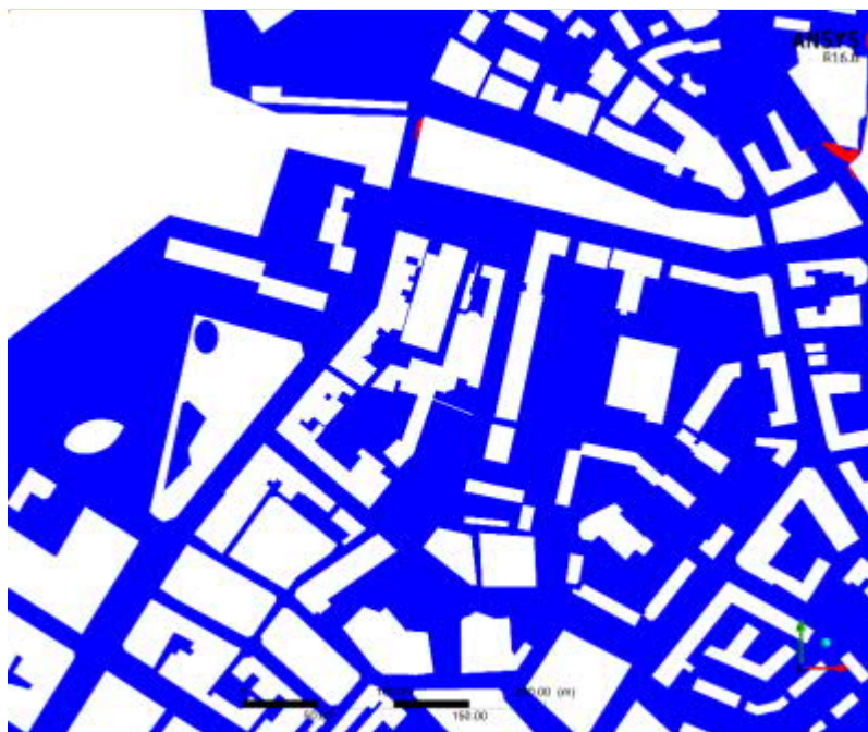
Figure 11-12 : Lawson 15m/s Distress for frail/elderly and cyclists - Existing. Red indicates unacceptable conditions.
