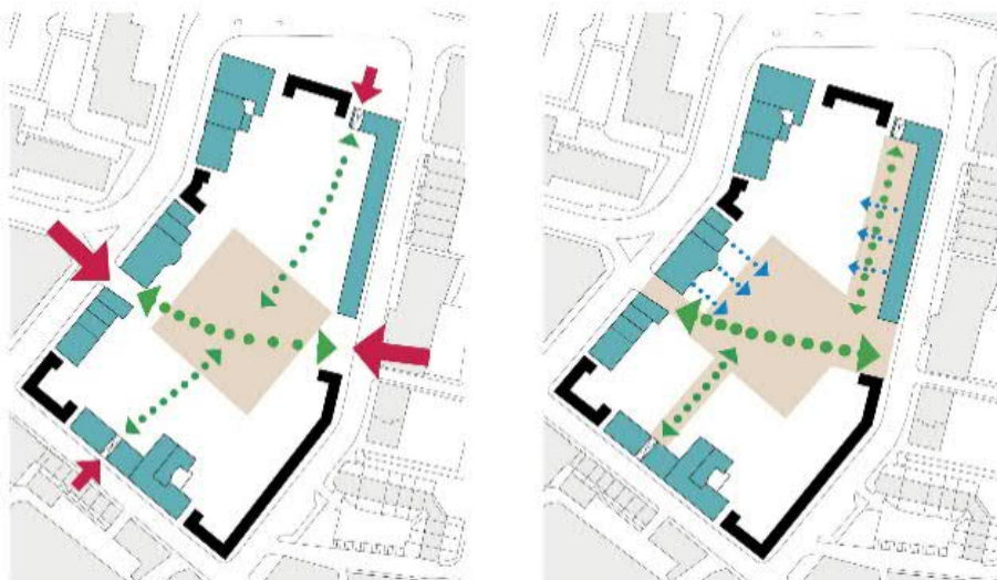
Figure 4.2 Establishment of a strong perimeter edge to the street and formation of internal spaces and relationships to important buildings
