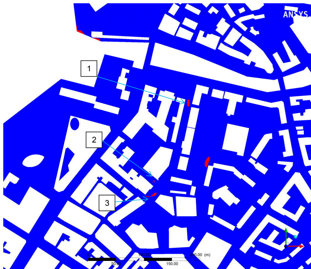
Figure 11-20: Lawson 15m/s Distress for frail/elderly and cyclists - Proposed development with mitigation. Red indicates unacceptable conditions.
